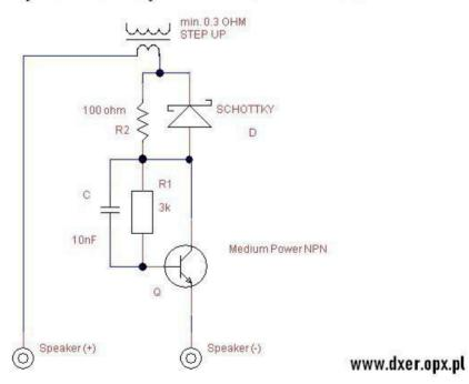
Alternatively, you can also use another circuit to match the impedance, or both at the same time, if we had a good transformer, but for some reason with a very low secondary winding resistance:
