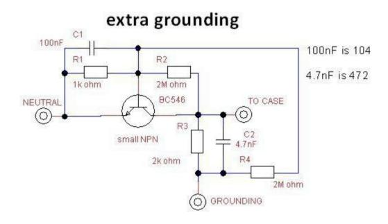
If our transformer - taken e.g. from a radio tape recorder - had an impedance of the secondary side (measured simply with an ohmmeter) below 1.5 ohms, we can successfully use a circuit called in Poland a 'dyne', and it looks like in the picture and is connected to the minus:
